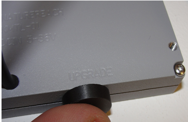
Figure 21. Positioning the earth magnet for firmware programming mode
