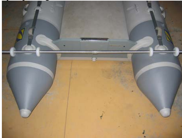
Figure 2. Adjusting the anti sway donuts
