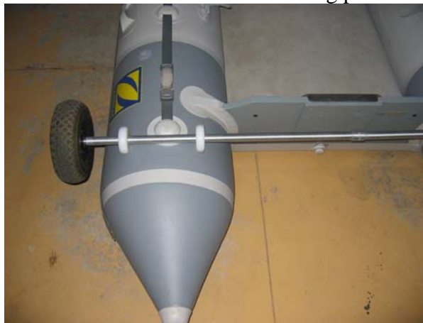
Figure 3. Installing the wheels
